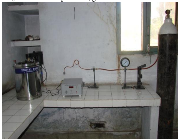
Fig 4.6: Bomb Calorimeter used for measurement of Calorific value [18]
