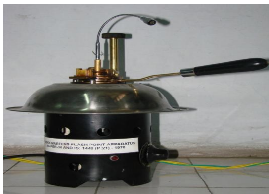
Fig 4.2: Pensky Marten apparatus used for measurement of flash and fire point [18]
